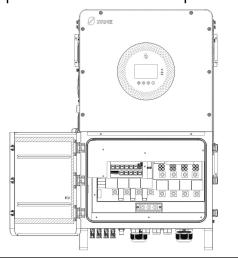
Wiring. (Note: The wire must be inserted into the corresponding connector before crimping the terminal.)
